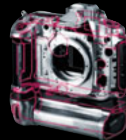
Enhanced moisture- and dust-resistant areas are outlined in red.
